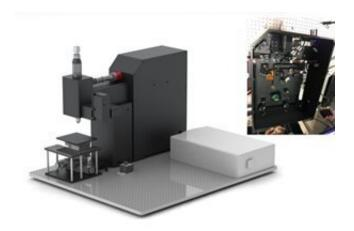
Researchers have developed a system that increases the imaging speed of two-photon microscopy up five times without compromising resolution. On the left, is a CAD model of the compact custom built two-photon microscopy system. The free-space optics inside is pictured on the right. Credit: Shih-Chi Chen from The Chinese University of Hong Kong
