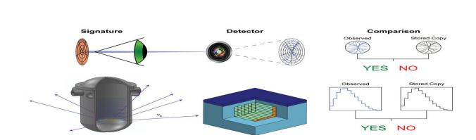
The principle of reactor operation verification with antineutrino monitors. The process for verifying reactor inventory integrity with antineutrinos bears similarities to biometric scans such as retinal identity verification. Credit: Georgia Tech
