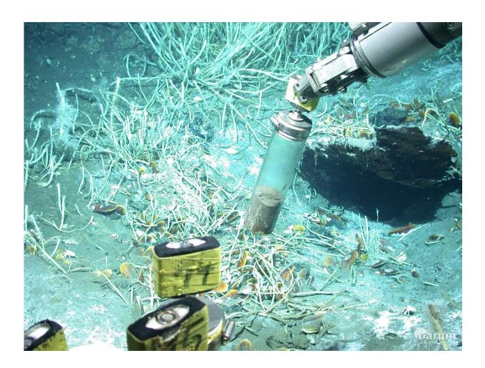
The submersible vehicle MARUM-QUEST samples for sediment at oil seeps in the Gulf of Mexico. Credit: MARUM -- Center for Marine Environmental Sciences
