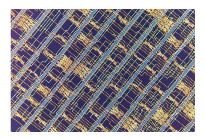
A close up of a modern microprocessor built from carbon nanotube field-effect transistors. Credit: Felice Frankel
