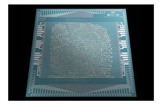
MIT engineers have built a modern microprocessor from carbon nanotube fieldeffect transistors (pictured), which are seen as faster and greener than silicon transistors. The new approach uses the same fabrication processes used for silicon chips. Credit: Massachusetts Institute of Technology
