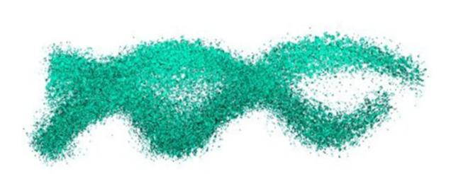
Simulated image of 3D twisted plasma wave structure (electron density perturbation) driven by the twisted or "corkscrew" laser waves. Credit: Yin Shi PhD, University of California San Diego
