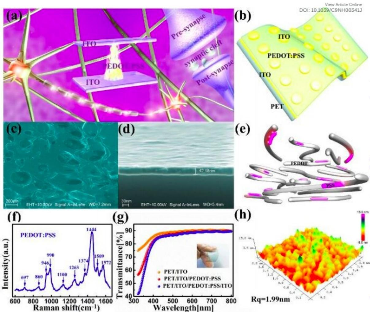
Structure and materials of the transparent and flexible synapses. a) Illustration of the identical bio-synapse and artificial synapse structures. The two electrodes and the functional layer correspond to pre-synapse, post-synapse, and synaptic
