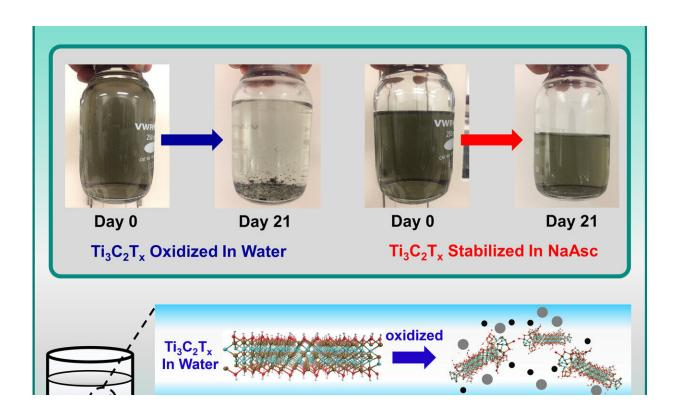
This graphic shows how a common MXene oxidizes, or degrades, under normal conditions, but is protected when exposed to a solution containing sodium L-ascorbate, a compound in the same family as vitamin C. Credit: Texas A&M University Engineering
