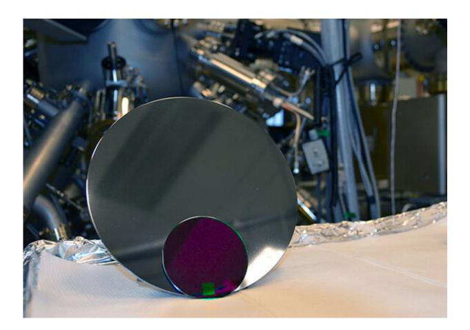
A 10 x 10mm chip (green) represents the conventional bulk oxide substrate. A 3-inch virtual oxide substrate on silicon(purple) is now possible. The 8-inch silicon wafer (silver) is projected for industry scale up. In the background is a hybrid molecular beam epitaxy system. Credit: MRI/Penn State
