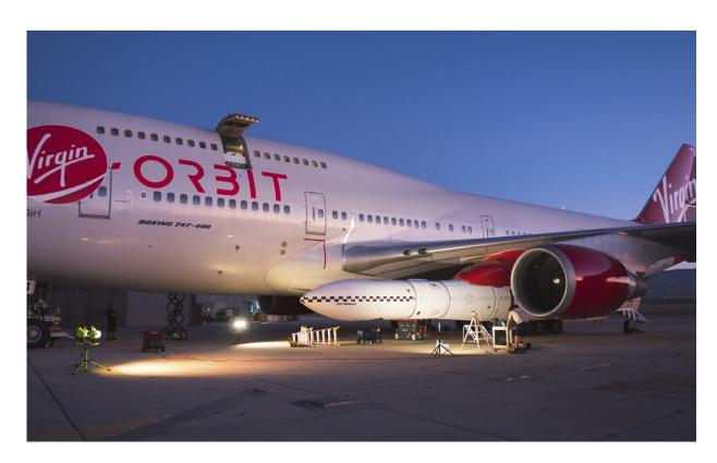
In this photo provided by Virgin Orbit, a rocket is shown attached to the wing of a Boeing 747 airplane on the tarmac of the Mojave Air and Space Port in Mojave, Calif, Wednesday, July 10, 2019, prior to a test flight during which the rocket was released from the airplane. The "drop test," which did not involve firing the rocket motor, was part of a test of Virgin Orbit's air-launched satellite booster, and is considered to be a key step toward space missions. (Greg Robinson/Virgin Orbit via AP)
