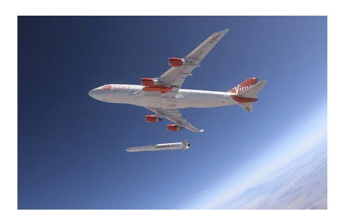
In this photo provided by Virgin Orbit, a rocket is dropped from a Boeing 747 airplane flying above Edwards Air Force Base in California, Wednesday, July 10, 2019. The "drop test," which did not involve firing the rocket motor, was part of a test of Virgin Orbit's air-launched satellite booster, and is considered to be a key step toward space missions. (Greg Robinson/Virgin Orbit via AP)
