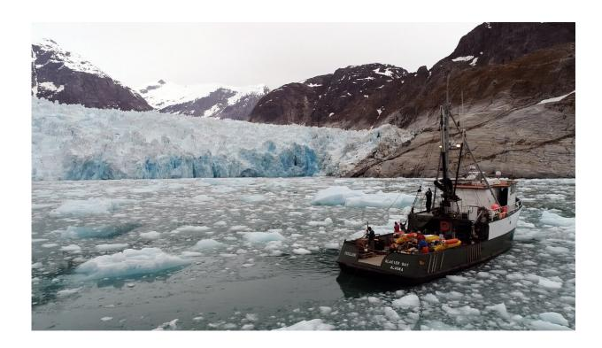
Researchers on the MV Steller are in front of the terminus of Alaska's LeConte Glacier in August 2016. An over-the-side pole holds the sonar instrument that collects data on the subsurface ice face as the vessel moves slowly through the icy water. Credit: David Sutherland
