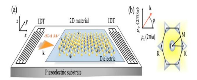
Two interdigital transducers (IDTs) generate and detect surface acoustic waves (SAWs, orange arrow). In-between the IDTs, these waves interact with the electrons of a 2D material, such as molybdenum disulfide (MoS2), giving rise to conventional and unconventional acoustoelectric currents. MoS2 is separated from the piezoelectric substrate by a dielectric layer. Credit: IBS
