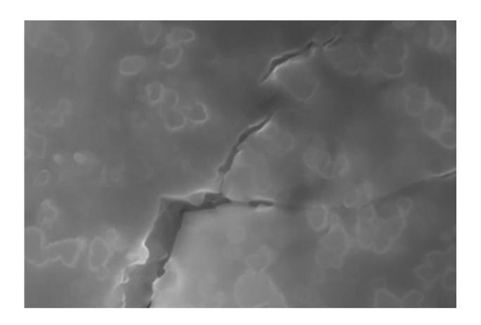
An electron microscope image of a new, tougher glass developed at UCLA, showing how nanoparticles (rounded, irregular shapes) deflect a crack and force it to branch out. Credit: SciFacturing Lab/UCLA
