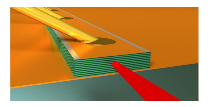
Schematic of one laser ridge in the thermoelectrically cooled THz quantum cascade laser. Credit: Faist group, ETH Zurich
