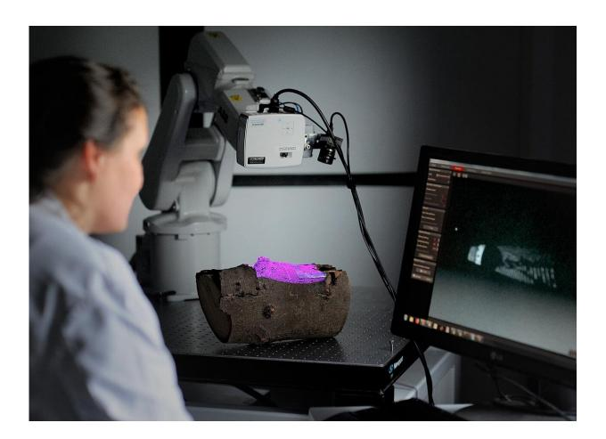
Researchers detected insect damage in wood samples using time-domain terahertz tomography performed with a robotic arm. Here, Kirsti Krügener is acquiring a reflection terahertz tomographic image measurement Credit: HAWK University of Applied Science and Arts
