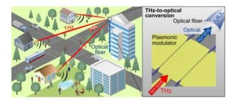
Seamless integration of wireless links into fiber-optical networks is the key to high-performance data networks: future cellular networks will consist of many small radio cells that can be connected flexibly by high-performance THz transmission links. At the receiver, THz signals can be converted directly into optical signals with the help of ultra-rapid plasmonic modulators and transmitted via glass fiber networks.
