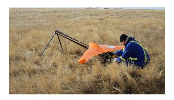
A fixed-wing UAV screening system being launched from a catapult. Credit: The Conversation
