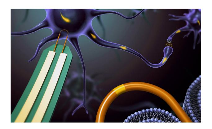
U-shaped nanowires can record electrical chatter inside a brain or heart cell without causing any damage. The devices are 100 times smaller than their biggest competitors, which kill a cell after recording. Credit: Lieber Group, Harvard University
