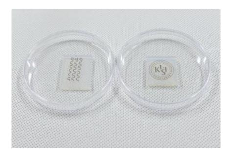
The real transfer-printing electrode that uses hydrogel and nano ink produced by Hyunjung Yi of the KIST's Post-Silicon Semiconductor Institute. Credit: Korea Institute of Science and Technology (KIST)
