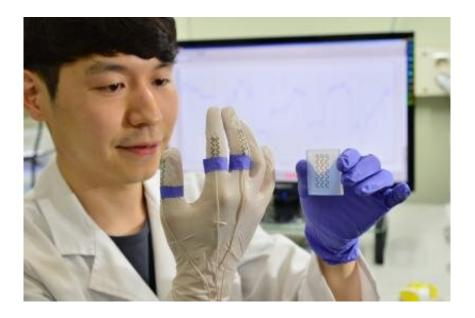
With the transfer-printing technology developed by researcher of KIST's Post-Silicon Semiconductor, they are conducting experiments to detect finger movements by implementing high-performance sensors on top of experimental gloves. Credit: Korea Institute of Science and Technology (KIST)
