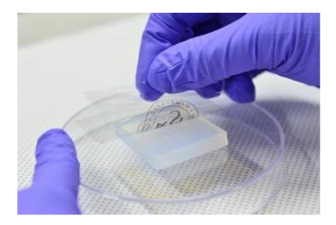
It is easily transferring electrodes on top of hydrogel (bottom) to PET film (top) with the transfer-printing technology that was developed by a researcher of KIST's Post-Silicon Semiconductor. Credit: Korea Institute of Science and
