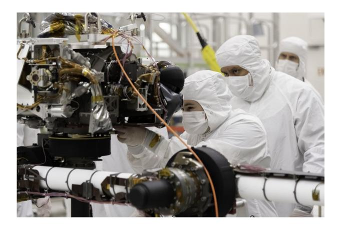
In this image taken on July 11, 2019, engineers at JPL install a sensor-filled turret on the end of the rover's 7-foot-long (2.1-meter-long) robotic arm. The turret includes HD cameras, the Scanning Habitable Environments with Raman & Luminescence for Organics & Chemicals (SHERLOC) science instrument, the Planetary Instrument for X-ray Lithochemistry (PIXL) science instrument, and a percussive drill and coring mechanism. Credit: NASA/JPL-Caltech
