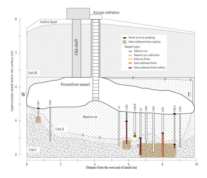
A schematic of the study site, which consists of a tunnel, excavated from a massive ice formation in the permafrost, and accessed through a narrow vertical opening. Researchers then drill below the tunnel floor to reach the cryopeg layer with its saline liquid (bottom hatched area). Credit: Shelly Carpenter/University of Washington
