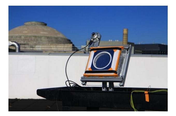
A test device installed on a rooftop at MIT proved the effectiveness of the new insulating material. When placed in sunlight the device heated up to 220 degrees C., even though the outside temperature at the time was about zero degrees.
