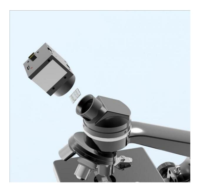
Schematic illustration on the location with the Smartlens is placed within the optical instrument (in this case a microscope). Credit: ICFO/ Marc Montagut
