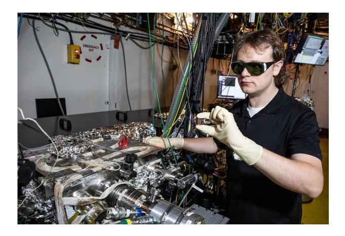
SLAC staff scientist Alexander Reid, the first user of the lab's instrument for ultrafast electron diffraction (MeV-UED) since it became available to the international community as part of the LCLS facility, handles an interchangeable sample card used to hold samples during UED experiments. Credit: Jacqueline Orrell/SLAC National Accelerator Laboratory
