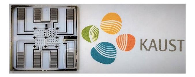
A thin-film chip with the energy-storing microsupercapacitors arrayed along top and bottom of the chip. Credit: KAUST
