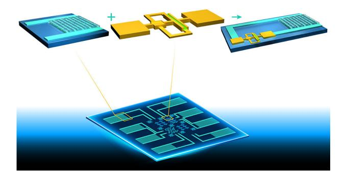
A schematic illustration of the integrated circuit fabricated on a one-inch glass substrate. The chip combines electronics and on-chip energy-storage units. Credit: WILEY-VCH Verlag GmbH & Co. KGaA, Weinheim
