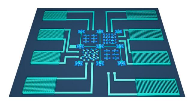
This illustration depicts on-chip electrochemical energy storage integrated with thin-film electronics at the transistor level using a single-electrode material for all devices. Credit: WILEY-VCH Verlag GmbH & Co. KGaA, Weinheim
