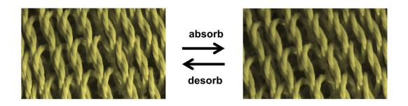
These photographs show the porosity increase of a knitted SRAM textile when exposed to water. This reversible porosity change enables evaporation of sweat. Credit: The University of Texas at Dallas
