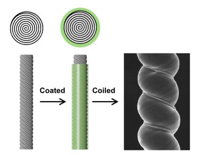
This illustration shows a twisted carbon nanotube yarn (CNT) (left) and a sheathrun artificial muscle (SRAM) made by coating a twisted CNT yarn with a polymer sheath. A scanning electron microscope image of a 42-micron outerdiameter coiled SRAM is shown on the right. Credit: The University of Texas at Dallas
