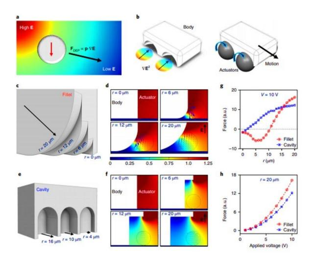
Spatial encoding of DEP attraction sites by modulating the 3D geometry. (a), A negatively polarized particle, with a lower relative permittivity than the medium ( $\epsilon p 0$ ) or away (F
