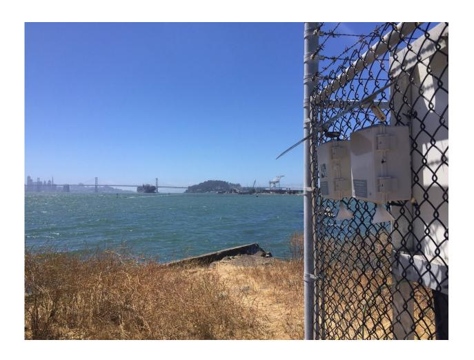
Two sensors in the largest black carbon air quality monitoring network ever deployed in a single city, with a spatial density approximately 100 times greater than traditional regulatory networks. The lowest black carbon levels were consistently recorded at sites like the one pictured, upwind of freeways and most industrial activity. Credit: Chelsea Preble/Berkeley Lab
