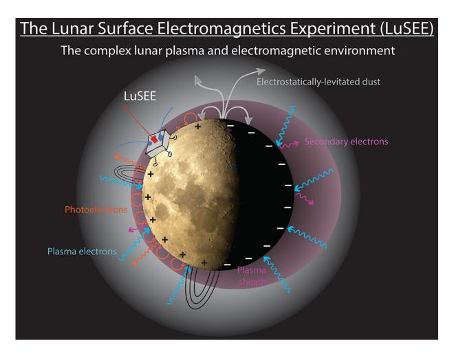
The Lunar Surface Electromagnetics Experiment, or LuSEE, will be built by the Space Science Laboratory to study the magnetic and electric fields on the moon's surface and how they interact with fine dust particles. The scientific instruments will land on the daylight side of the moon, where sunlight knocks electrons our of atoms to electrostatically charge and levitate the dust. Credit: Stuart Bale
