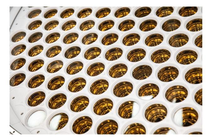
An intricately thin wire grid is visible (click image to view larger size) atop an array of photomultiplier tube. The components are part of the LZ inner detector. Credit: Matt Kapust/SURF
