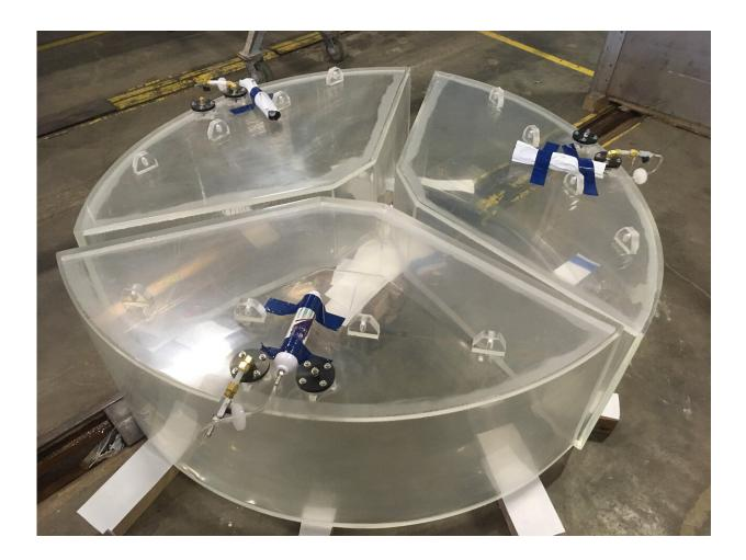
The bottom three acrylic tanks for the LUX-ZEPLIN outer detector during testing at the fabrication vendor. These tanks are now at the Sanford Underground Research Facility in Lead, South Dakota. Credit: LZ Collaboration
