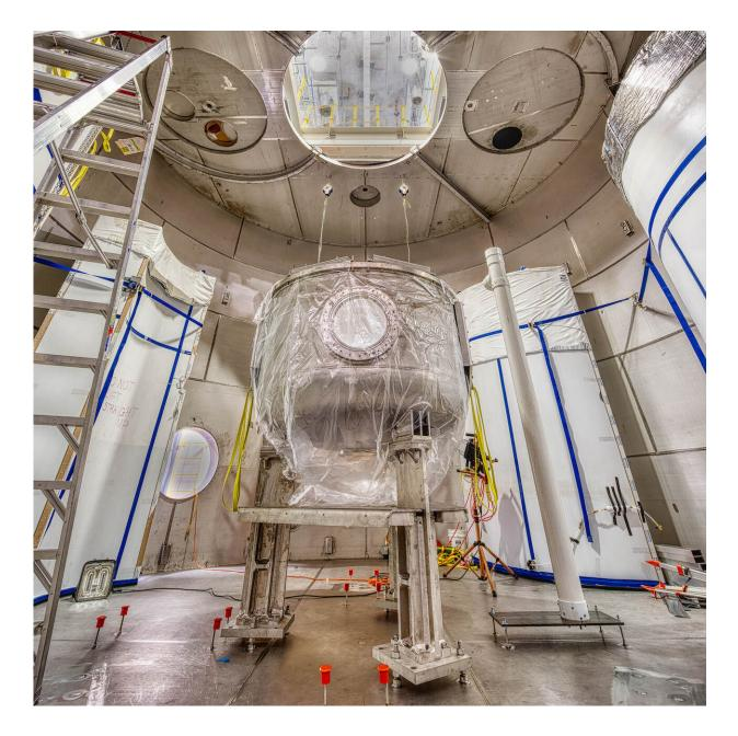
Components for the LUX-ZEPLIN project are stored inside a water tank nearly a mile below ground. The inner detector will be installed on the central mount pictured here, and acrylic vessels (wrapped in white) will fit snugly around this inner detector. Credit: Matt Kapust/SURF
