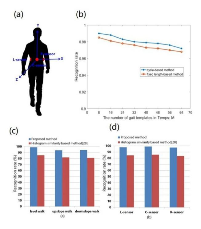
(a) Placement of acceleration sensor nodes; (b) Impact of the number of templat es in Temps on recognition rate; (c) and (d) Comparison of identity recognition of older adults using the proposed method. Credit: Dr. Sun Fangmin)
