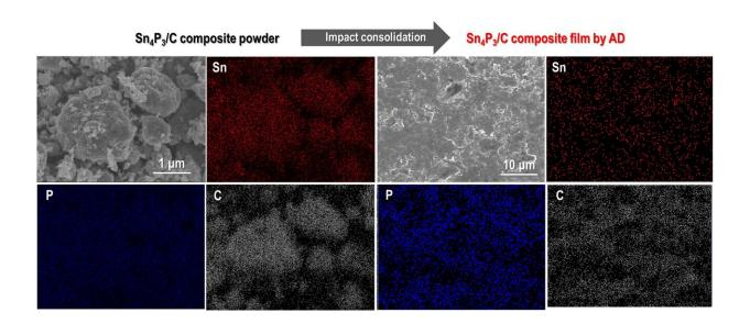
Scanning electron microscope (SEM) images of Sn4P3/C composite particles (1st row:1st image), and surface of Sn4P3/C composite film fabricated by the AD process (1st row:3rd image). Corresponding elementary distributions for Sn, P, and C are also shown. Credit: (c) Toyohashi University of Technology. All Rights Reserved.
