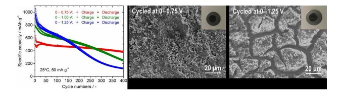
Long-term cycling performance of Sn4P3/C composite films at different cell voltage windows ranging from 0 V to 0.75 V, and that from 1 V and to 1.25 V (left). SEM images of Sn4P3/C composite film surfaces cycled at 0 V-0.75 V (middle) and that at 0 V-1.25 V (right) are also shown. Credit: (c) Toyohashi University Of Technology.
