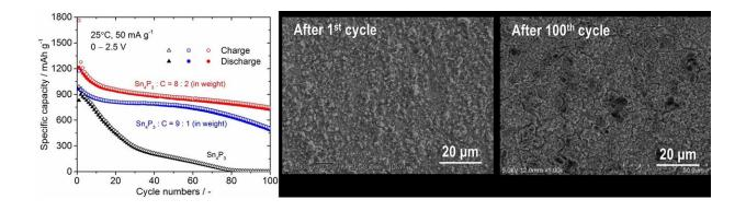
Cycling performance of  $Sn_4P_3$  and  $Sn_4P_3/C$  composite films for different carbon contents (left) in a two-electrode cell with Li metal as the counter electrode. Cycling test was performed at cell voltage windows ranging from 0 V to 2.5 V. SEM images of  $Sn_4P_3/C$  composite film surface after the 1st (middle) and  $100_{th}$ cycles (right) are also shown. Credit: (c) Toyohashi University of Technology. All Rights Reserved.
