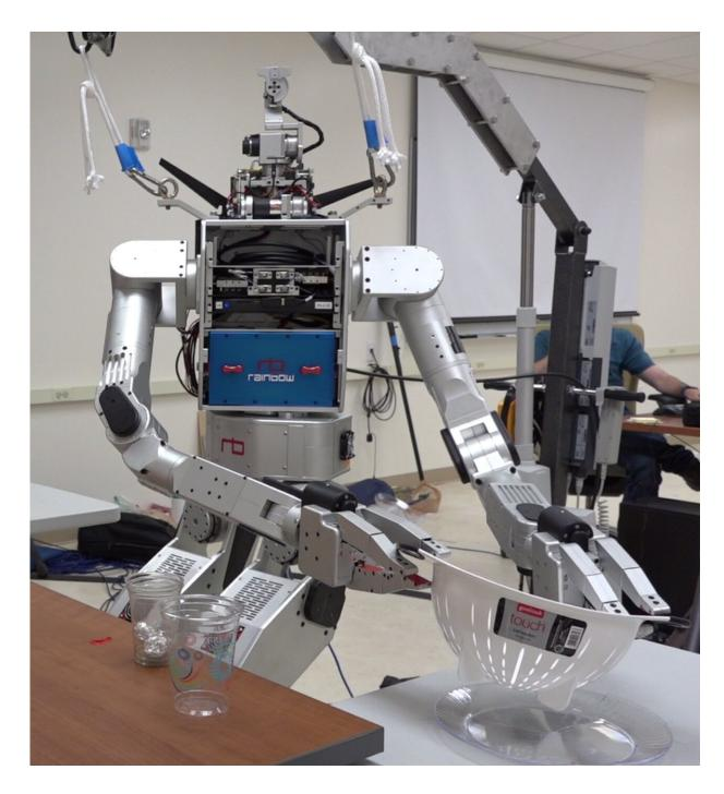
A connected robot reaches for a colander in Bilge Mutlu's UW–Madison lab, where studies have made robots better at working with remote human controllers. Credit: Bilge Mutlu
