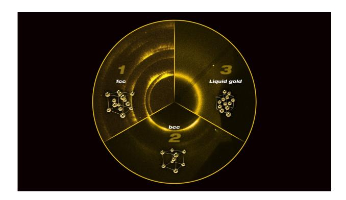
Three of the images collected at Argonne National Laboratory's Dynamic Compression Sector, highlighting diffracted signals recorded on the X-ray detector. Section 1 shows the starting face-centered cubic structure; Section 2 shows the new body-centered cubic structure at 220 GPa; and Section 3 shows the liquid gold at 330 GPa. Credit: Lawrence Livermore National Laboratory
