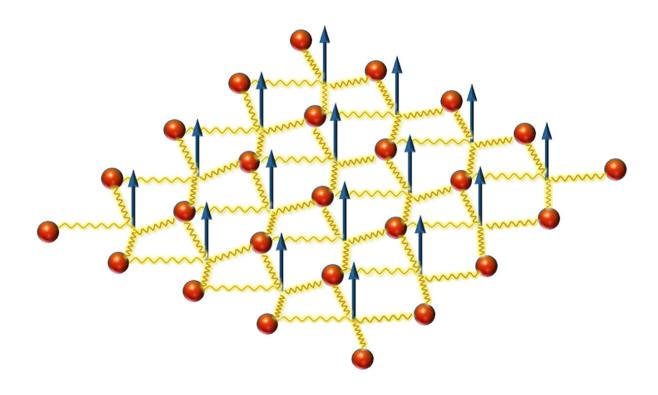
Electrons in a 2D lattice interact with a magnetic field (blue perpendicular arrows), and its quantum fluctuations via the exchange of photons (wiggly yellow lines), which changes how the electrons move through the lattice. Credit: Vasil Rokaj
