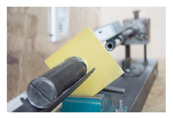
A compact acceleration test bench was used for studying the ballistic properties. During the experiment, a ballistic stand was placed inside the testing machine for stretching the sample to the given value of preliminary load. Speed of the projectile varied from 100 to 800 m/s for each level of loading.
