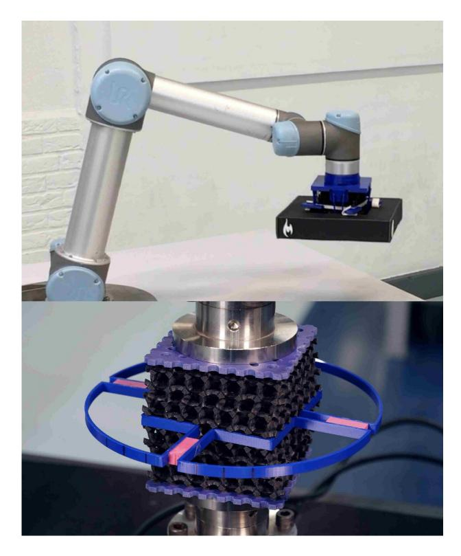
A conventional robotic arm is modified using the developed soft actuators to provide soft touch during pick-and-place tasks. Credit: Delft University of Technology
