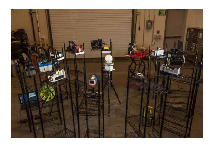
Emerging semiconductor sensors that can improve equipment used for detecting and identifying radioactive materials. Credit: Pacific Northwest National Laboratory
