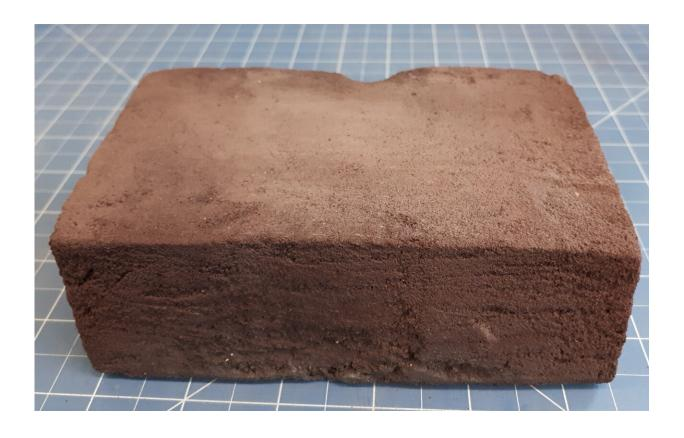
Artificial regolith brick. Credit: ESA/Azimut Space
