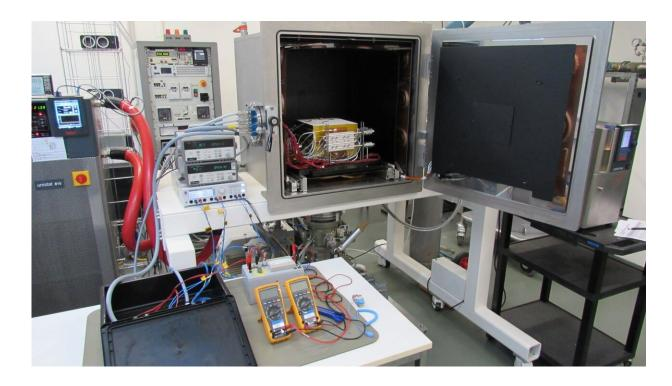
Artificial regolith brick in a vacuum chamber. Credit: ESA/Azimut Space
