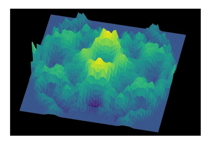
A 3-D representation of the spin-excitation continuum—a possible hallmark of a quantum spin liquid—observed in a single crystal sample of cerium zirconium pyrochlore in experiments at Oak Ridge National Laboratory (ORNL). Inelastic neutron-scattering experiments at ORNL's Spallation Neutron Source revealed spin-excitation continua in samples of cerium zirconium pyrochlore that were cooled as low 35 millikelvin. (Image by Tong Chen/Rice University) Credit: Tong Chen/Rice University
