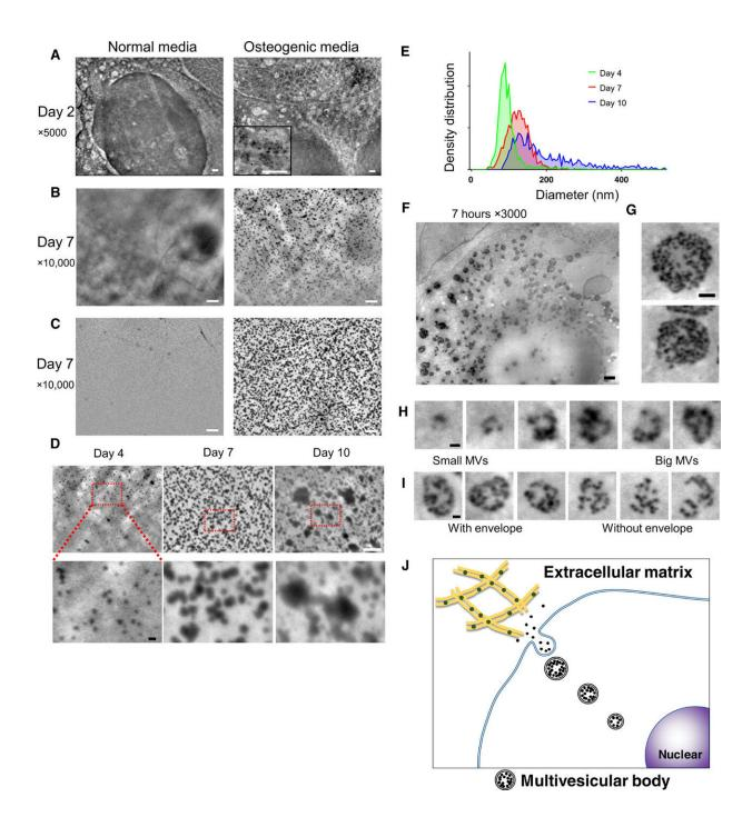
Nanoscale observation of live osteoblasts in culture media, using the SE-ADM system. (A) Representative high-resolution SE-ADM images of osteoblasts
