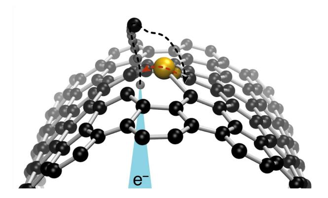
An electron beam focused on a carbon atom next to a silicon impurity atom within the curved wall of a single-walled carbon nanotube can controllably make it jump to where the beam was placed. Credit: © Toma Susi/University of Vienna
