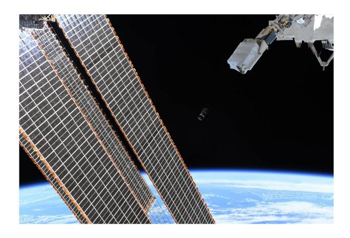
SpooQy-1 was ejected from the Japanese Small Satellite Orbital Deployer past the International Space Station's (ISS) solar arrays. This photograph was taken by an astronaut on the ISS. Credit: NASA
