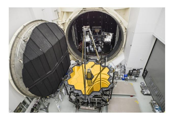
NASA's "Chamber A," an enormous thermal vacuum testing chamber housed at NASA's Johnson Space Center in Houston was previously used to test Apollo moon mission hardware and on occasion, suited astronauts. Chamber A saw extensive upgrades to properly support tests of Webb's revolutionary hardware. Credit: NASA/Chris Gunn
