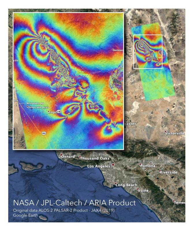
NASA's Advanced Rapid Imaging and Analysis (ARIA) team created this coseismic Interferometric Synthetic Aperture Radar (InSAR) map, which shows surface displacement caused by the recent major earthquakes in Southern
