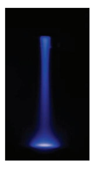
This particle beam polishes the surface of a new X-ray optic made of silicon. Credits: Chris Gunn/NASA
