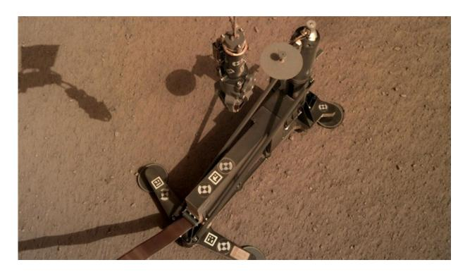
The Heat Flow and Physical Properties Package deployed on the Martian surface. Image Credit: NASA/DLR
