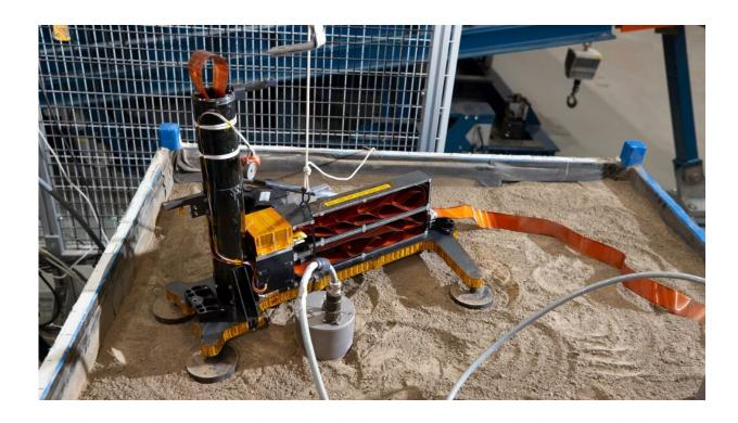
The HP3 model in its test bed in Bremen. Image Credit: DLR.
