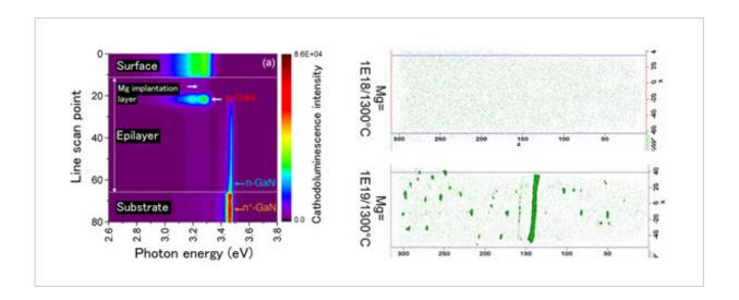
Results of cathodoluminescence analysis applied to Mg ion-implanted GaN (left) and three-dimensional distribution of Mg atoms introduced into GaN as visualized by atom probe tomography (right). Credit: NIMS
