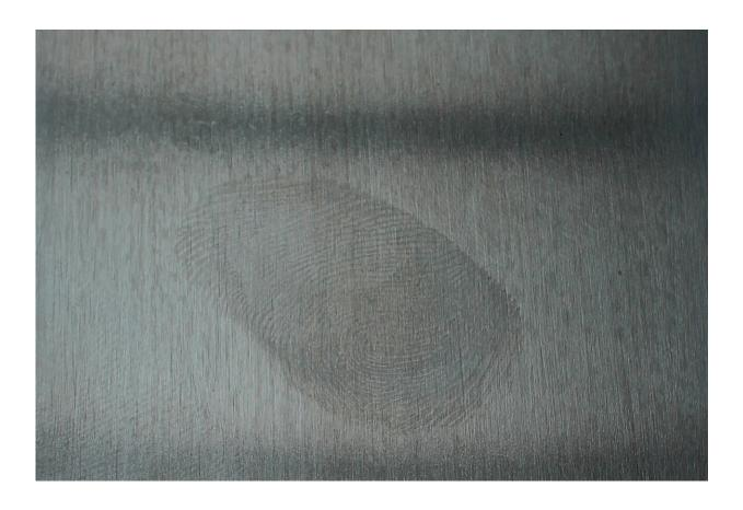
The new sol/gel nanocoating is designed to prevent fingerprints on stainless steel and metal surfaces. Credit: Fraunhofer IMWS
