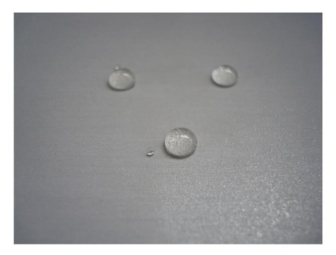
Drops of oil on a super hydrophobic and oleophobic coating on stainless steel. Credit: FEW Chemicals GmbH Wolfen
