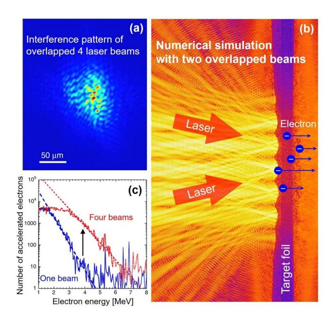
Efficient high energy electron generation by interfering multiple laser beamlets.
