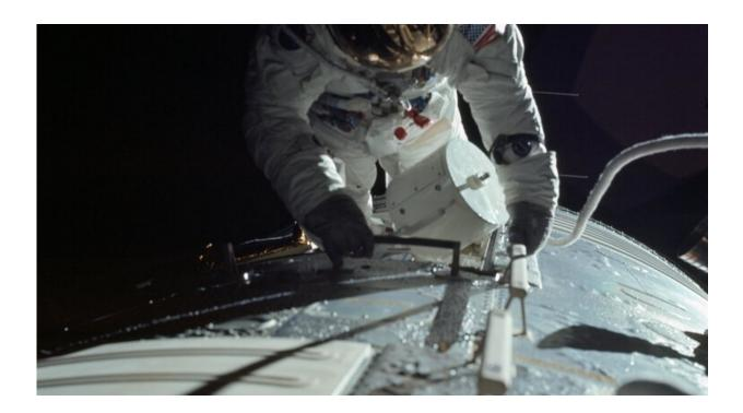
Apollo 17 astronaut Ron Evans had to embark on a spacewalk just to retrieve a cassette of film, which recorded data from the first radar mapping instrument mounted on a spacecraft. Credit: NASA
